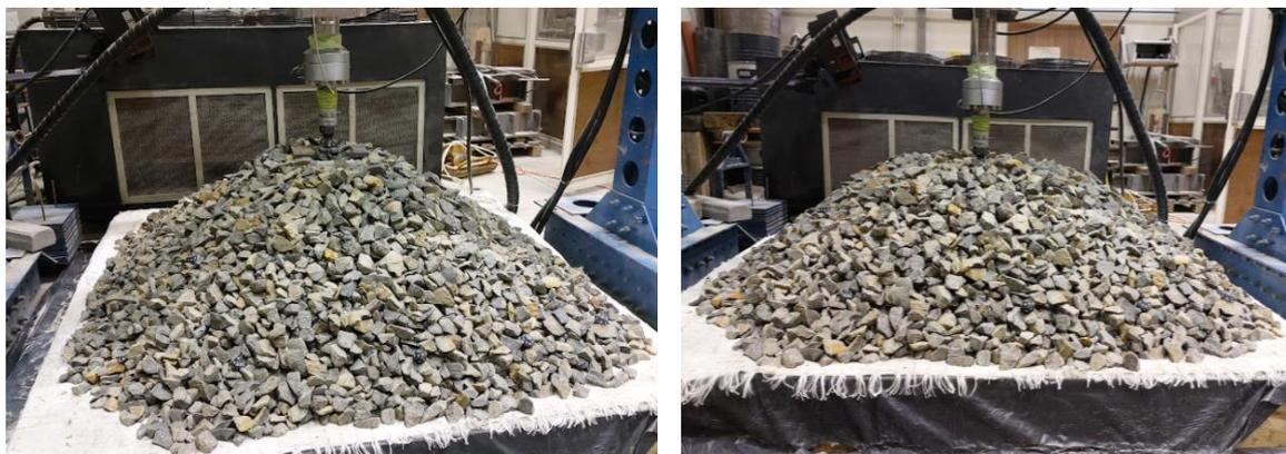
**Figure 10.** Photos of the laboratory sample before (left-hand side) and after loading (right-hand side)
