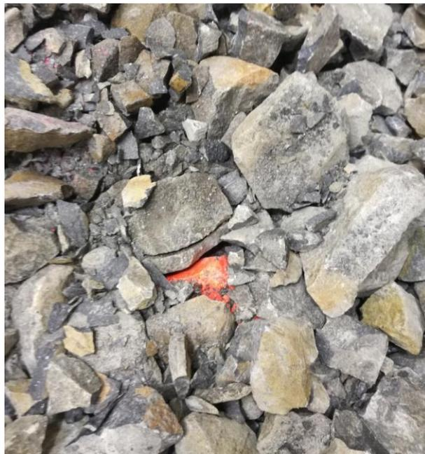
**Figure 31.** *Orange #1* stone in the fragmented, broken ballast
