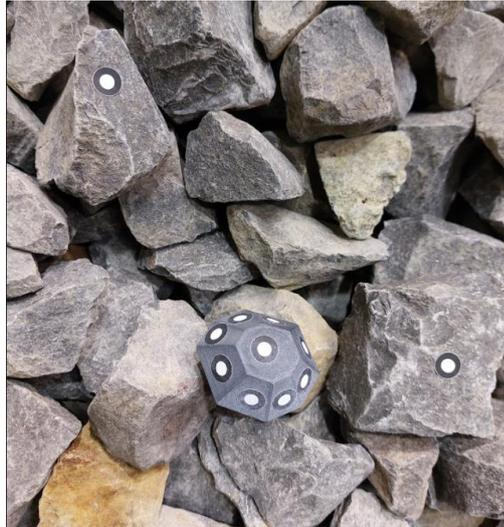
**Figure 9.** The 3D printed plastic body (i.e., “eikosi-tessera-eder”) with point stickers
