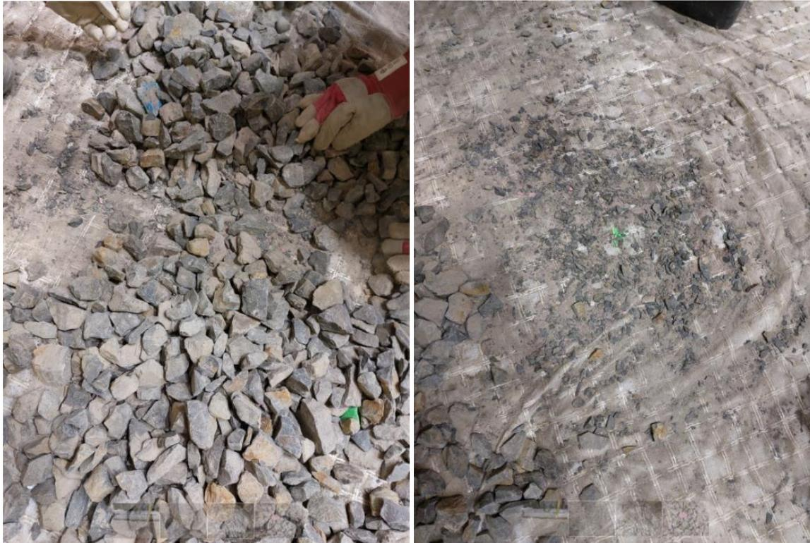
**Figure 36.** Dust and broken stone particles found in the lower layers
