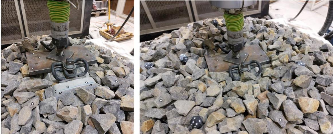
**Figure 11.** Photos of the sleeper piece before (left-hand side) and after loading (right-hand side)
