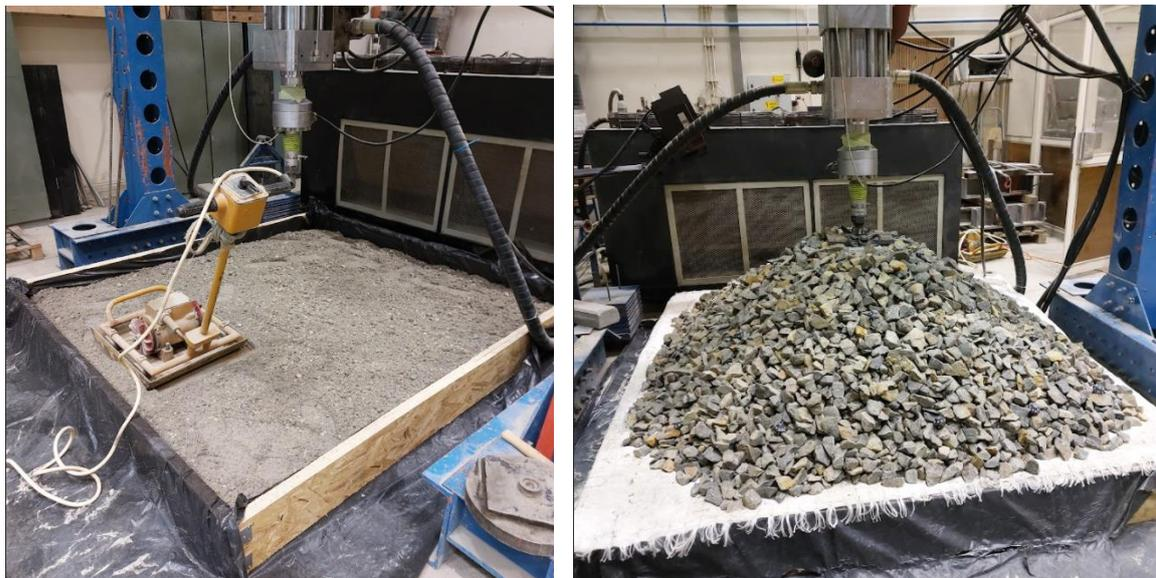
**Figure 4.** The test set-up: compacted sandy gravel layer on under ballast mat (left side); the constructed ballast bed part (right side)
