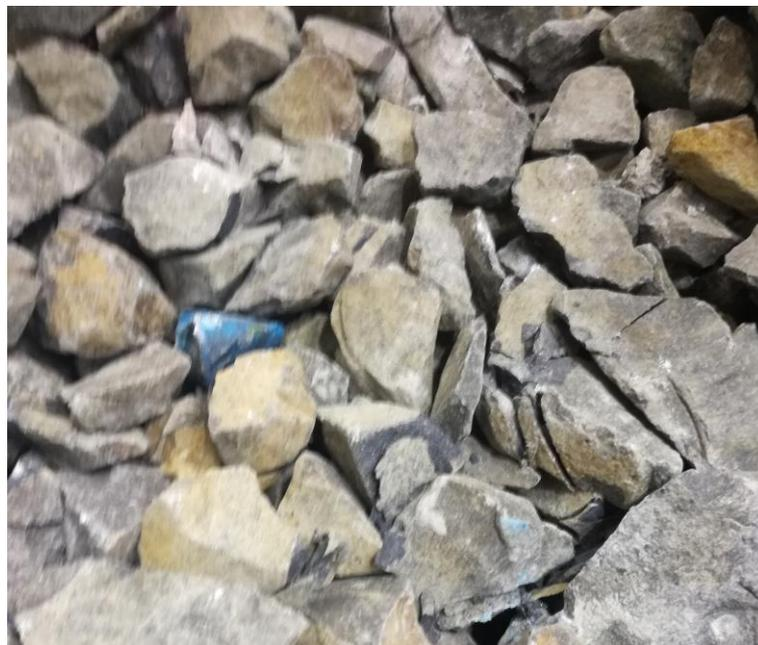
**Figure 26.** *Blue #1* stone in the fragmented, broken ballast (i.e., after the loading test)
