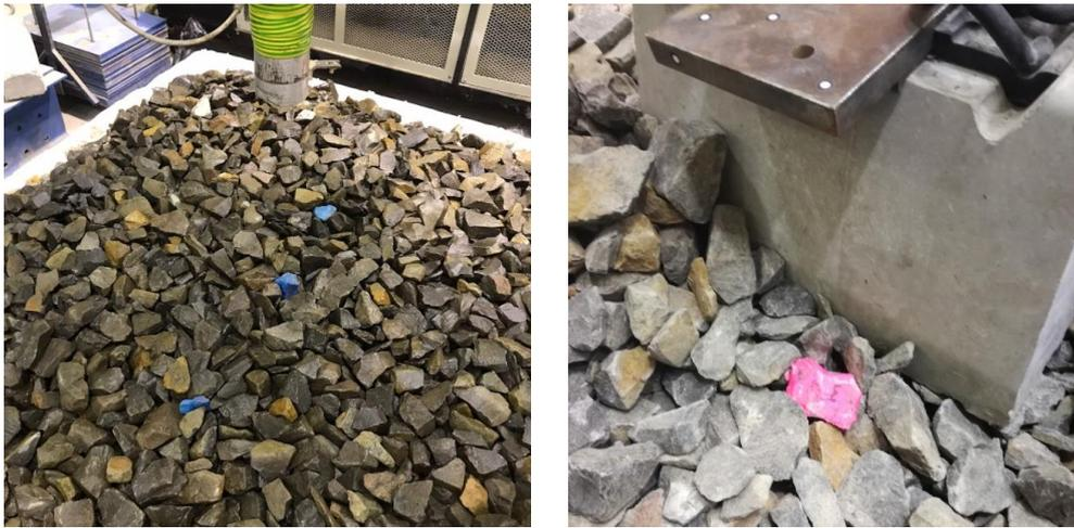
**Figure 5.** The ‘hidden’ and scanned colored elements in the ballast
