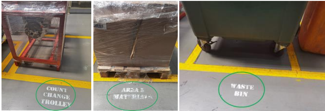
Figure 4. Improvement in demarcation.
