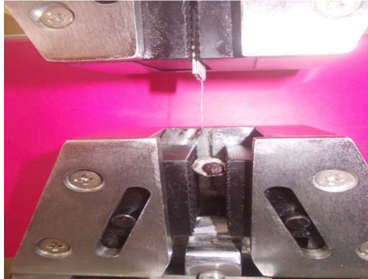
Figure 7. K11V test piece mounted on the testing machine (before traction)
