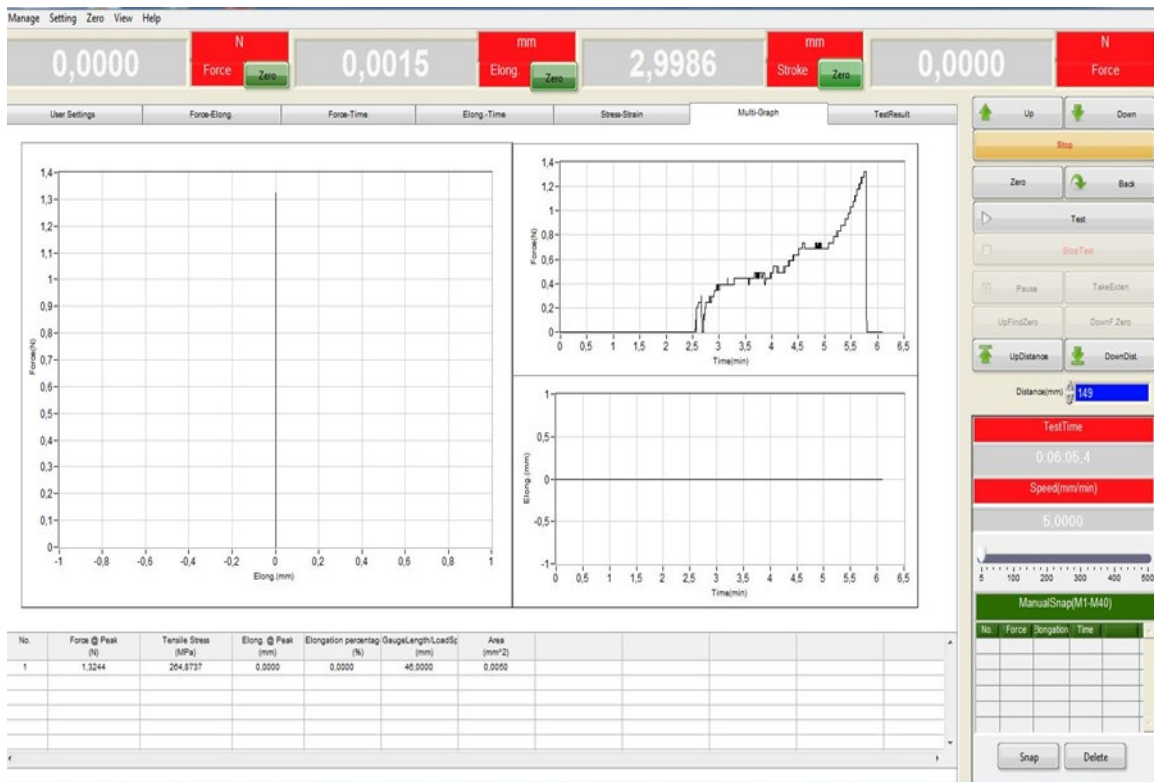
Figure 8. Result of fiber breakage after pull out
